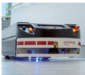
TRANSCAR Automated guided vehicle for voluminous goods transport.
